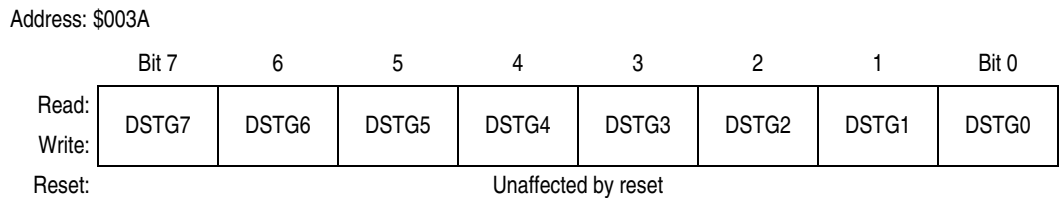
Figure 6-15. ICG DCO Stage Register (ICGDSR)
